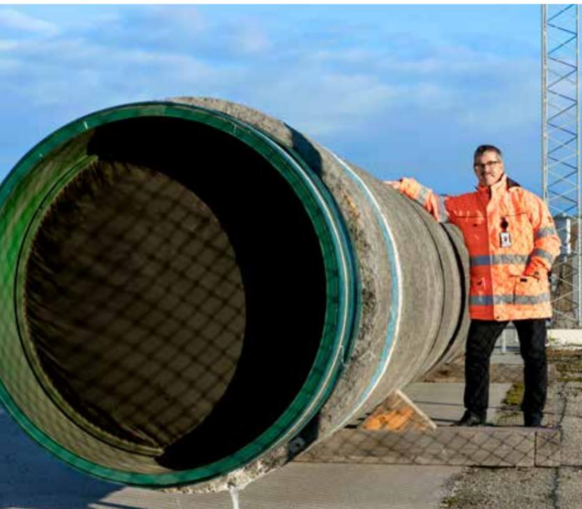
The pipes in the 1,200 km pipeline are 12.2 metres long, have an outer diameter of approximately 1,300 mm, an inner diameter of 1.153 mm and weigh up to 24 tonnes each. 30,000 of the total of 200,000 pipes are planned to go via the Port of Karlshamn.
